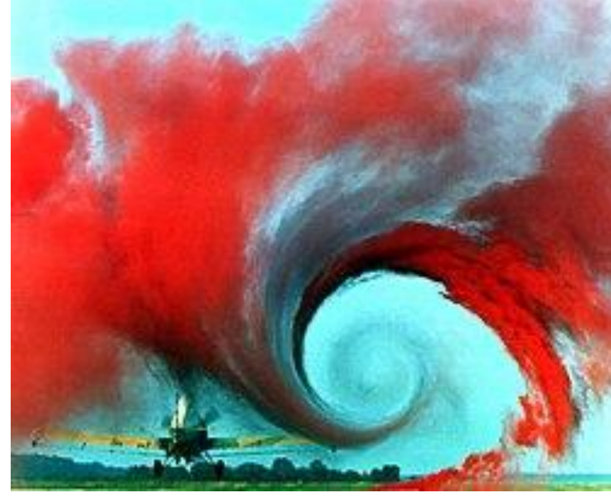
Aircraft wake turbulence 4 Scale: \sim 100 m, Re: \sim 10^7
