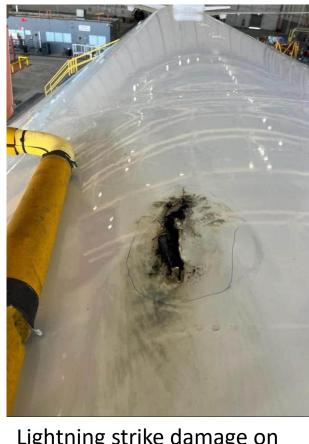
Lightning strike damage on an American Airlines Boeing 787 en route to Dallas, TX.
