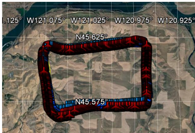
Figure 7.1: RV-12 HiL unit data flash logs (yellow line), ADS-B (blue aircraft) and LAMS position data (red aircraft).
