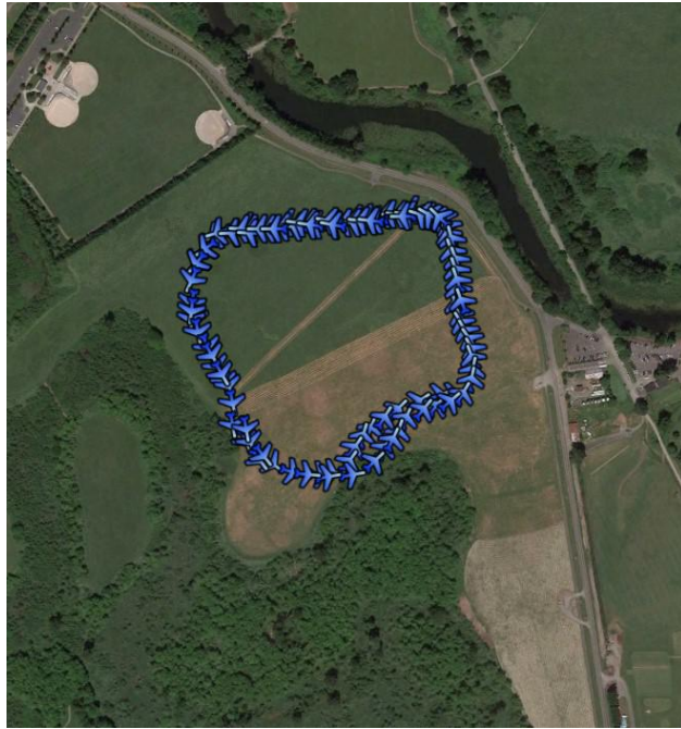
Figure 6.10: Initial test ADS-B position tracking results.
