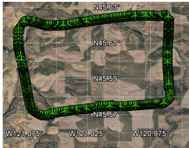
Figure 7.8: RV-12 fused (green aircraft) position estimates overlaid on data flash log track (yellow line).
