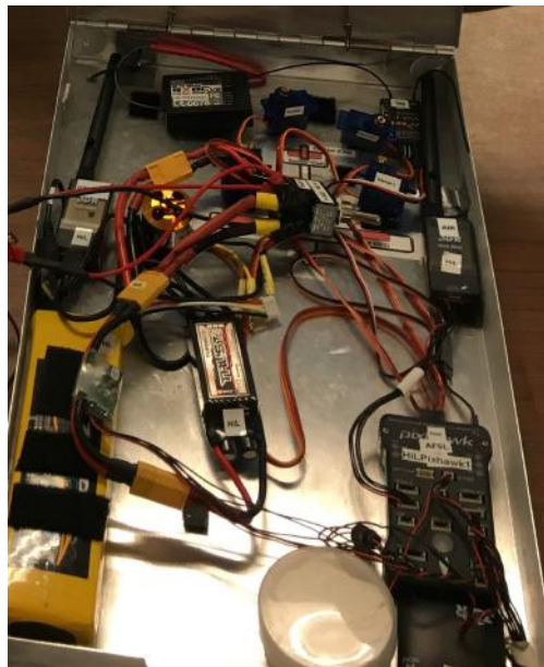
Figure 3.5: Secondary GPS HiL unit.
