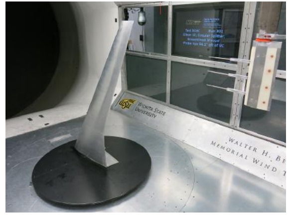
(b) Wake survey system installed in tunnel behind model.
