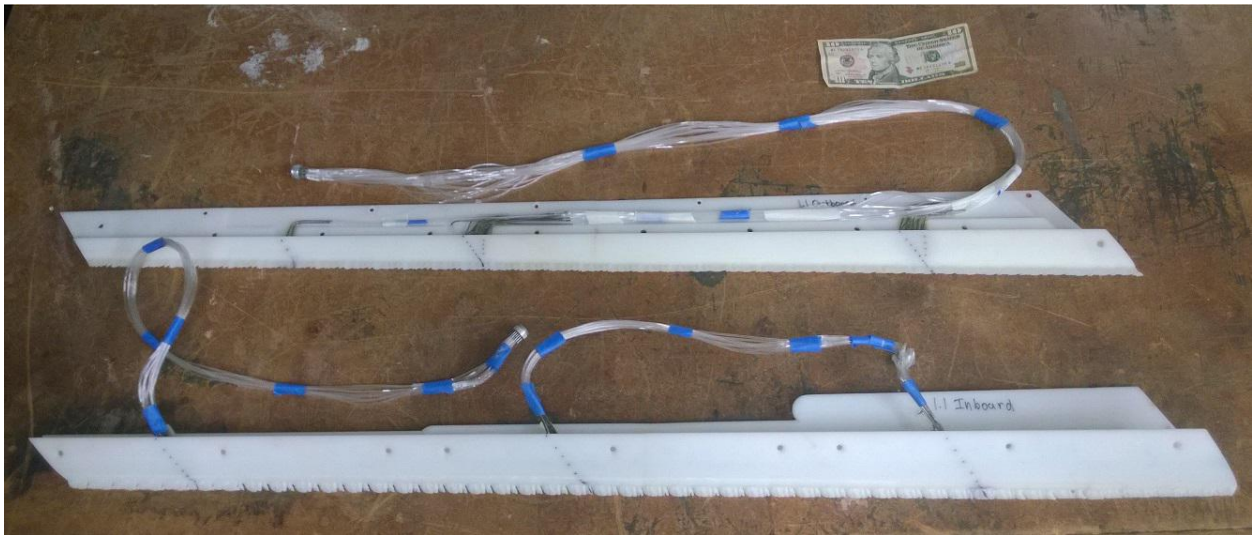
Figure 3. A fully instrumented ice shape of the maximum scallop configuration. Notice that the complete ice shape is broken into an inboard and outboard shape.
