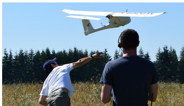
(b) Performing a hand launch of the CONDOR UAV.
