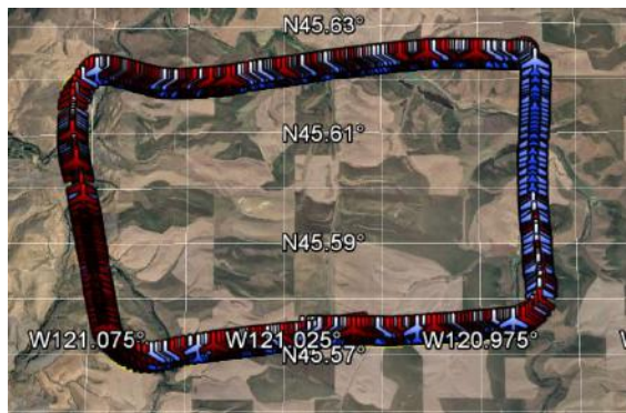
(a) RV-12 ADS-B raw (blue aircraft) and estimated (red aircraft) positions overlaid on data flash log track (yellow line).
