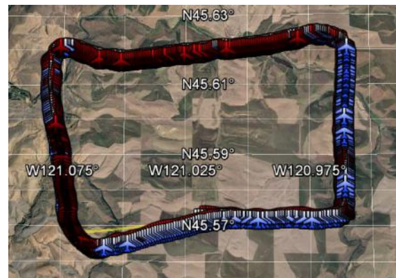
(b) RV-12 LAMS raw (blue aircraft) and estimated (red aircraft) positions overlaid on data flash log track (yellow line).
