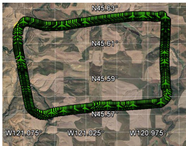
Figure 14. RV-12 fused (green aircraft) position estimates overlaid on data flash log track (yellow line).
