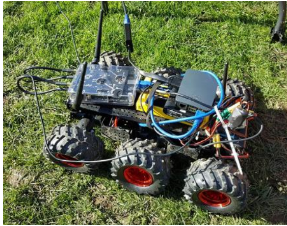
(a) Vehicle with SDR components for ground testing.
