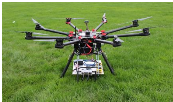
(c) DJI S1000+ “Argo” with SDR payload.
