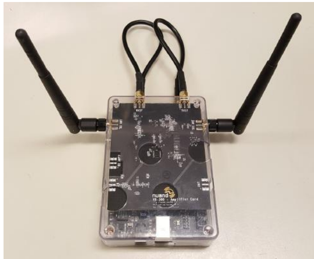
Figure 1. The BladeRF SDR board with the attached dipole antennas.
