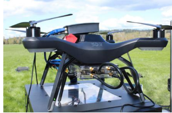
(b) 3D Robotics Solo with SDR payload.
