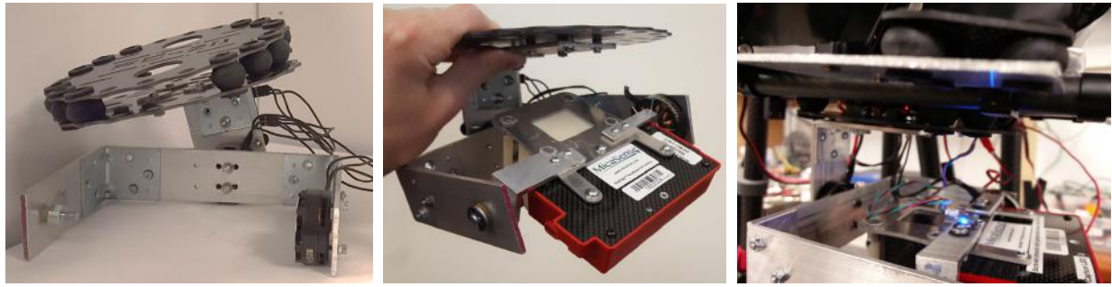
Fig. 8. Final MAPSS setup showcasing the final product utilized in this paper. The left image displays the dampening plate and structure without the Fixture Plate, FLIR Plate, and sensors installed. The center image shows MAPSS with the RedEdge and a 3D printed model of the FVPR installed. The right image shows MAPSS fully operational and mounted on the UAV used for testing on the right.
