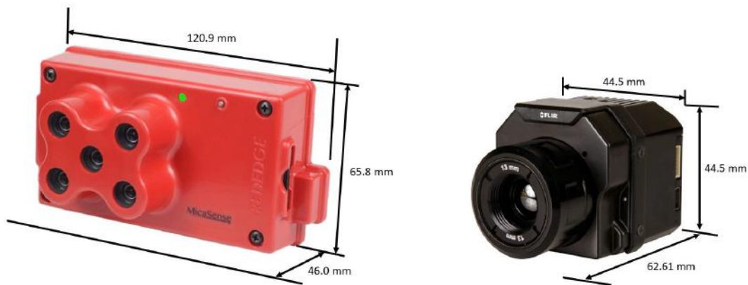
Fig. 1. The two sensors that will be attached to the gimbal system. On the left is the MicaSense RedEdge 9 and on the right is the FLIR Vue Pro R. 10 The dimensions include the length, height, and width (including protruding lens).
