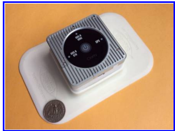
(b) Sagetech Corp. Clarity ADS-B in receiver.
