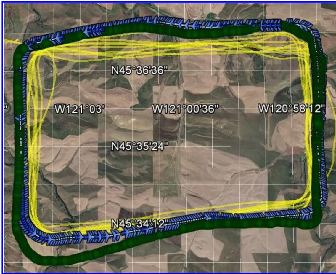
Figure 11. RV-12 Data. Data flash logs (yellow), ADS-B (blue planes), LAMS (green circles). TRAPIS (ADS-B and LAMS) recorded approximately 11.5 minutes of data where as HiLPixhawk1 (data flash logs) record approximately 2 hours of data (observe the RV-12 entering and exiting pattern in the upper left).
