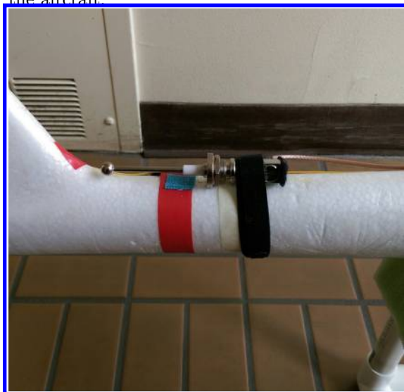
(a) ADS-B antenna in original orientation.
