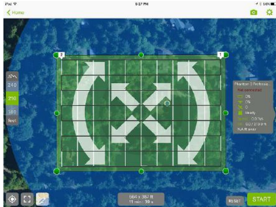
(a) Planning data acquisition using the Pix4DCapture app with a double grid pattern.
