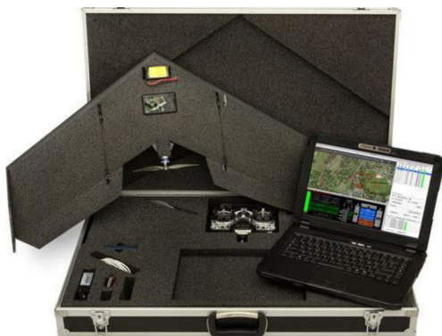
Figure 1. Swinglet UAS consisting of the aircraft, camera, GCS and manual control unit. Image from of SenseFly.com.
