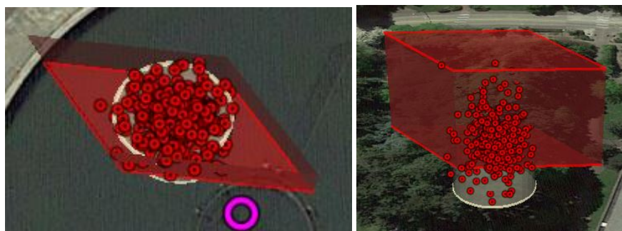
Figure 4.17: ACCV scenario 10, Monte Carlo simulation results top view (left) and side view (right)
