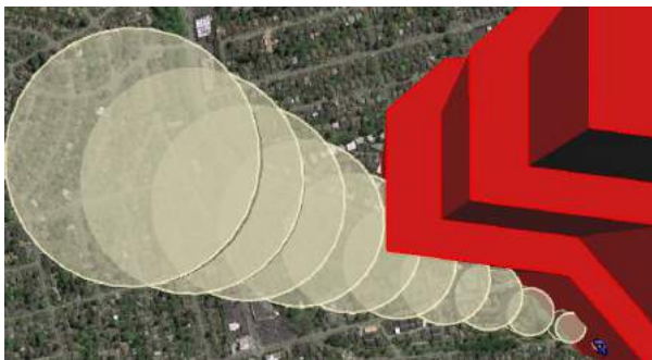
Figure 37. This is a top view of simulation 2's FSE results at 40 seconds. This is the xy-plane view clearly showing Prop13 violating the airspace at 40 seconds.
