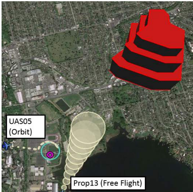
Figure 31. This is a top view of simulation 2's FSE results at 0 seconds. Furthermore the initial FSE results between UAS05 and Prop13 are within close proximity and the aircraft conflict calculator predicts conflicts between these two aircrafts for the next 14 seconds.
