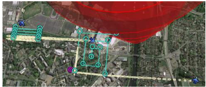
Figure 28. This is a top view of simulation 1's FSE results at 45 seconds. In addition to switching the flight path of UAS06, the UAS06's operator relinquishes command of UAS06 after sending UAS06 back to the parallel track. Next the operator changes perspective entity and controls UAS04. This operator then switches UAS04's flight mode from free flight to following the expanding square flight path.
