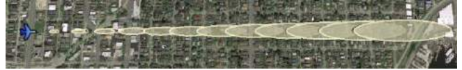
Figure 2. This shows an FSE free flight results from the top. Notice that errors in the initial velocity estimate will lead to larger regions in the body x-axis whereas errors in the initial flight path heading angle will yield larger propagation in the body y-axis.
