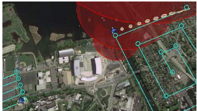
Figure 29. This is simulation 1's FSE results at 81 seconds. At this time the airspace conflict calculator determines UAS04 is currently violating the airspace.
