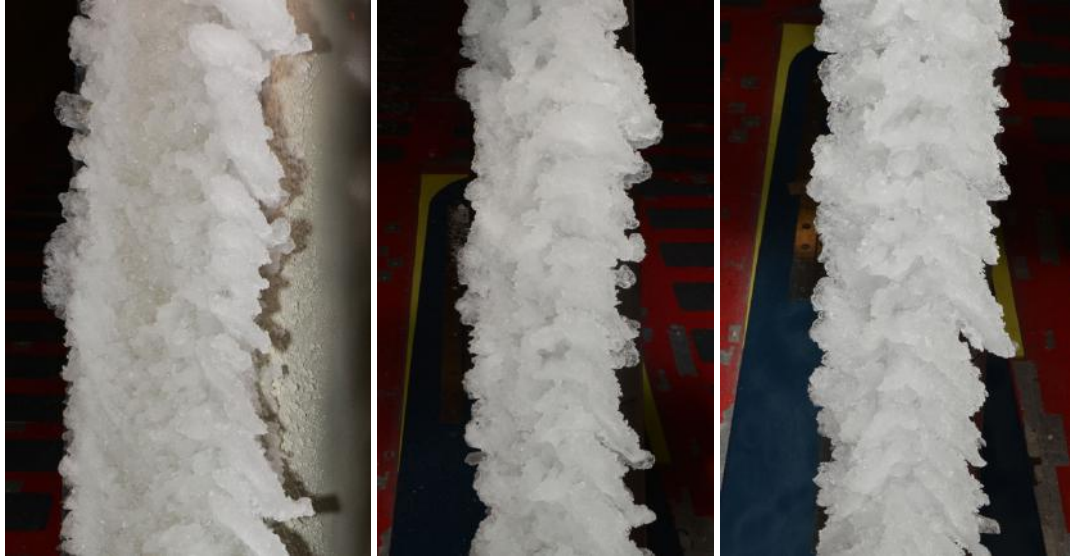
Figure 8. Run ID 23(“WB33”): Inboard, Midspan, and Outboard model ice accretions, respectively.
