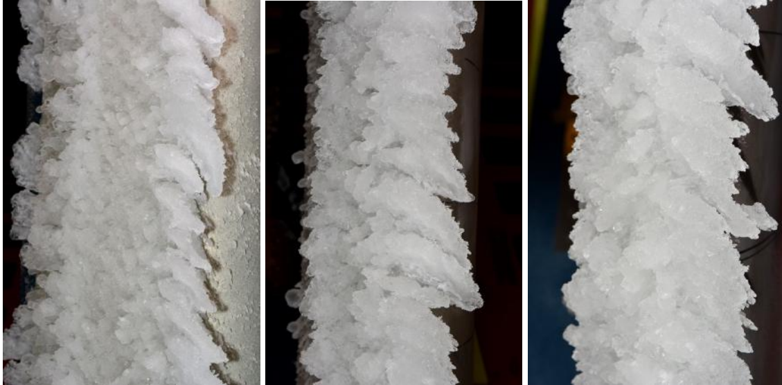
Figure 2. Run ID 3 ("Venetian Blind"): Inboard, Midspan, and Outboard model ice accretions, respectively.
