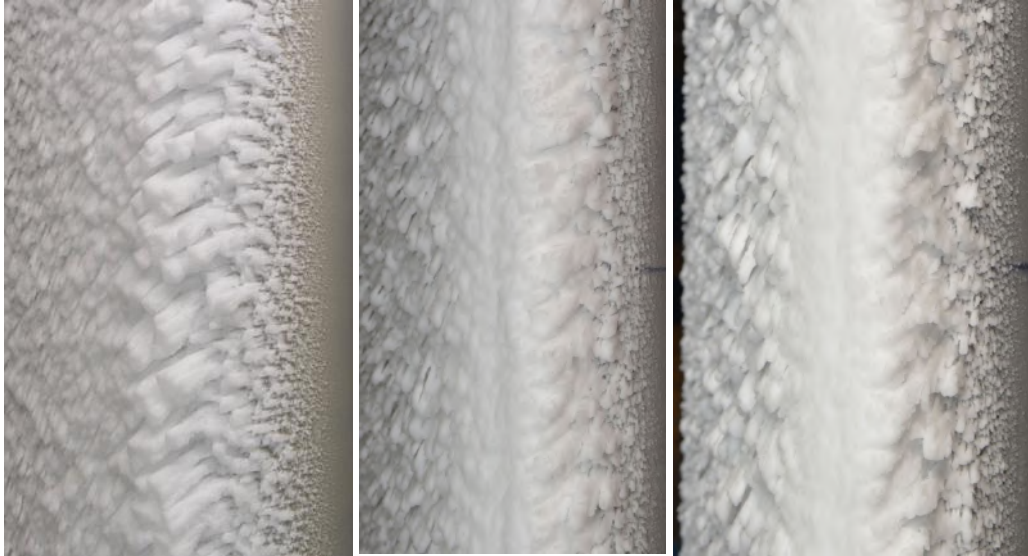
Figure 6. Run ID 9 ("Streamwise/Rime"): Inboard, Midspan, and Outboard model ice accretions, respectively.
