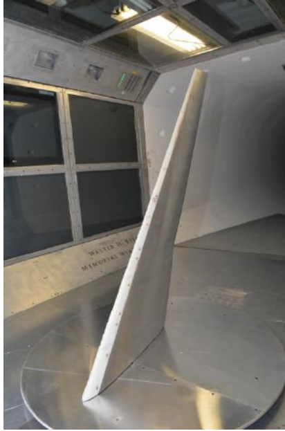
Figure 26. Rapid prototyped iced leading edge on the 8.9% CRM65 wind tunnel model.
