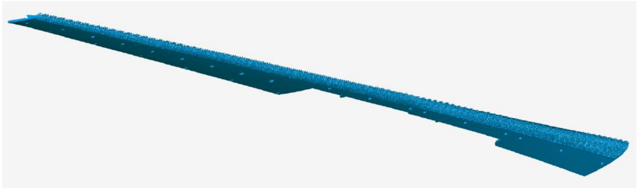
Figure 24. High-fidelity ice shape merged with the 8.9% subscale CRM65 removable leading edge.
