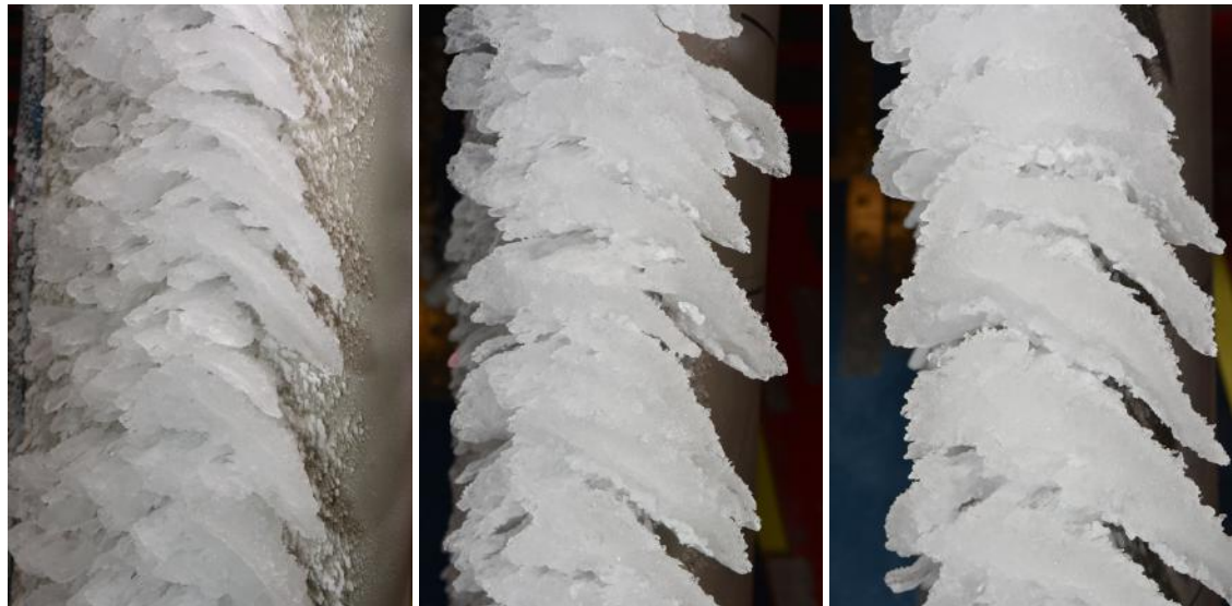
Figure 3. Run ID 4 ("Maximum Scallop"): Inboard, Midspan, and Outboard model ice accretions, respectively.
