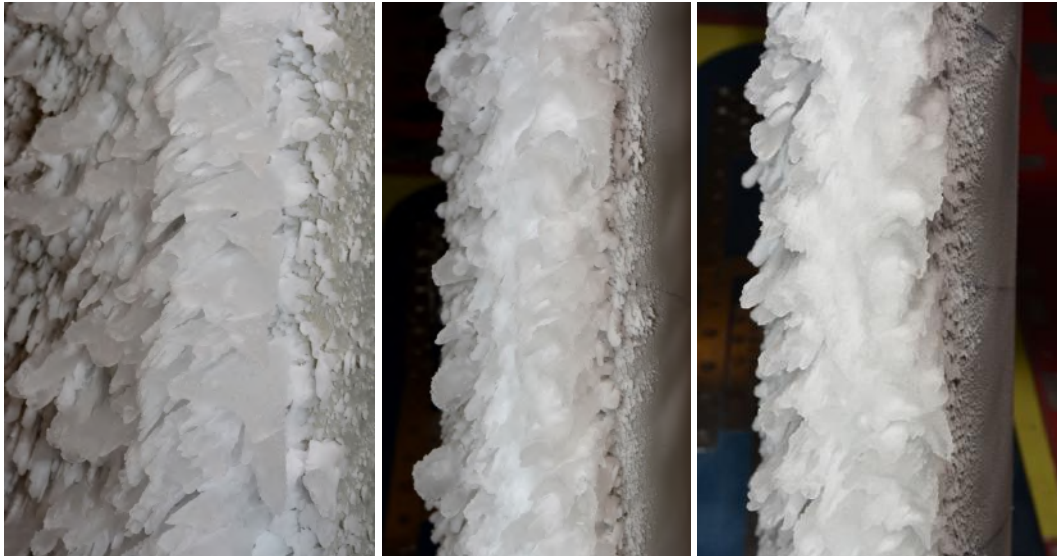
Figure 5. Run ID 6 ("Incomplete Scallop"): Inboard, Midspan, and Outboard model ice accretions, respectively.
