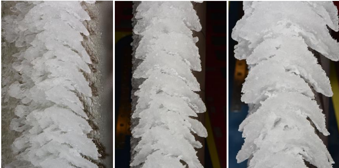
Figure 7. Run ID 22("Maximum Scallop Low AoA"): Inboard, Midspan, and Outboard model ice accretions, respectively.
