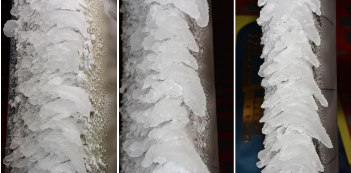
Figure 4. Run ID 5 ("Small Gap"): Inboard, Midspan, and Outboard model ice accretions, respectively.
