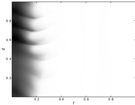
Figure 3: Ion density for the two-fluid model for the axisymmetric Z-pinch after 1.75 Alfvén transit times. The lower hybrid drift instability is observed. The two-fluid time steps are about  $1 \times 10^{-3}$ .
