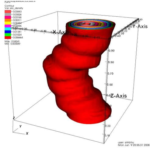
Figure 6: Ion density for Hall-MHD for the 3-dimensional Z-pinch with a kink instability perturbation after 2 Alfvén transit times. The lower hybrid drift instability is observed.
