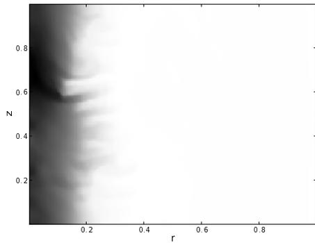
Figure 4: Ion density for Hall-MHD for the axisymmetric Z-pinch after 1.75 Alfvén transit times. The lower hybrid drift instability is observed. The Hall-MHD time steps are about  $2 \times 10^{-5}$ .
