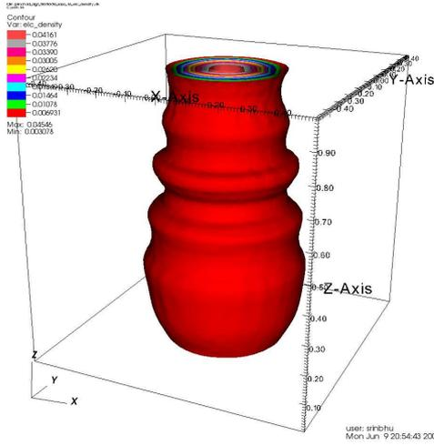
Figure 5: Ion density for the two-fluid model for the 3-dimensional Z-pinch with a sausage instability perturbation after 2 Alfvén transit times. The lower hybrid drift instability is observed.
