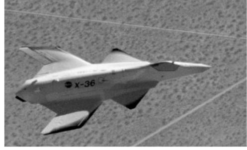
Fig. 1. Boeing/McDonnell Douglas X-36 tailless fighter agility research aircraft.
