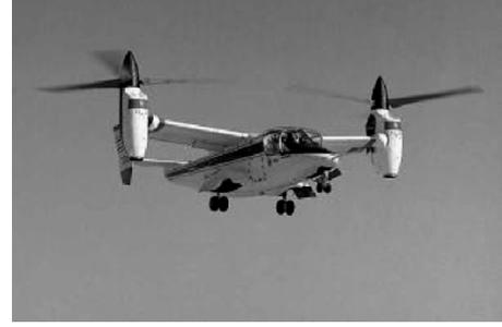
Fig. 3. XV-15 tilt-rotor in helicopter configuration.
