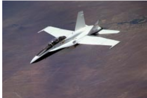
Fig.18. F-18 System Research Aircraft proposed for future upgrades, including damage adaptive flight control.
