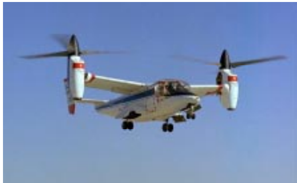
Fig. 1. XV-15 in helicopter configuration.
