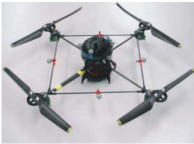
Fig. 15. Quadrotor vehicle equipped with reference markers.
