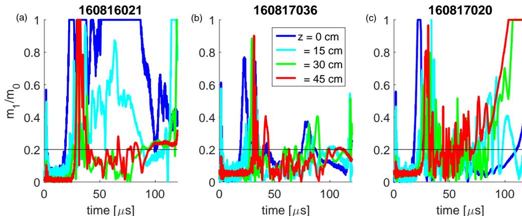
Figure 5.2: Normalized magnetic mode data,  $m_1/m_0$ , showing stability initially improves with increased compression bank voltage and then degrades at high voltages. Compression bank voltages of (a) 0 kV, (b) 2 kV, and (c) 8 kV are shown for pulses with otherwise identical run settings. Horizontal black lines indicate a current centroid displacement of 1 cm.
