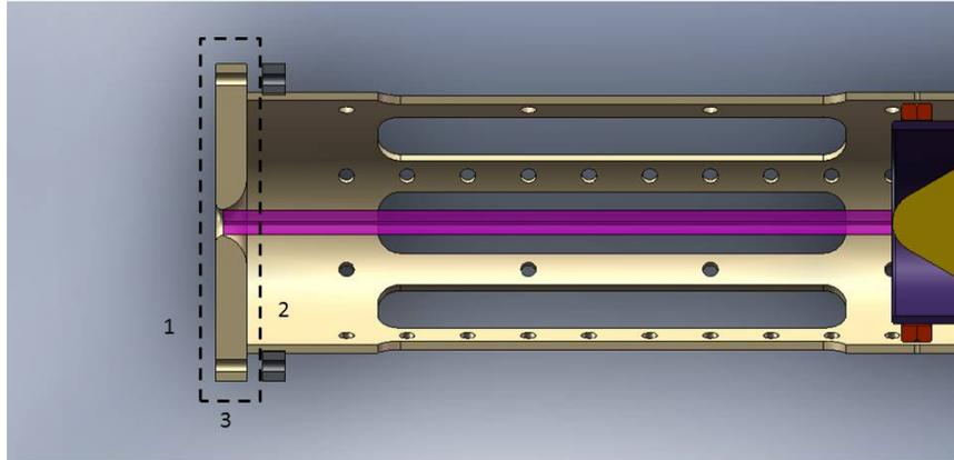
Figure D.3: A cylindrical control volume encompassing the endwall is used to solve for the net force on the endwall in the worst case.
