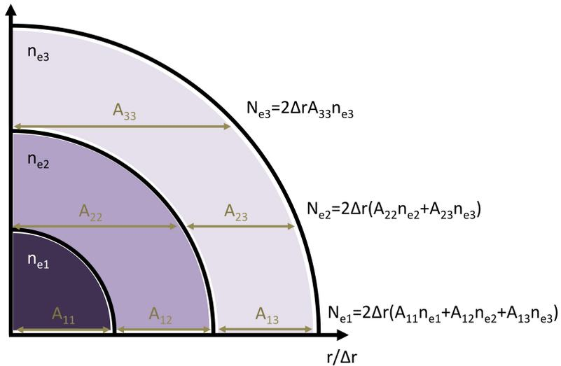
Figure 3.3: The Abel transform breaks up an axisymmetric plasma into concentric annular areas. Assuming uniform  $n_e$  in each annulus makes computation of  $N_e$  a matter of multiplying the discrete  $n_e$  by a matrix  $\mathbf{A}$  containing the relative lengths of chord lengths in the geometry. The elements of  $\mathbf{A}$  for a coarse discretization are shown here.  $\mathbf{A}$  can be expanded to arbitrary size to transform arbitrarily large  $n_e$  profiles.
