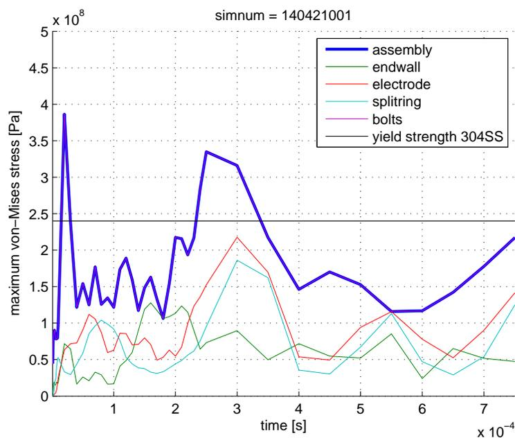
Figure D.8: The max von Mises stresses in each component of the single hole endwall assembly exhibit damped oscillations in time. Stresses before  $100 \mu s$  are caused by bolt pre-tension.
