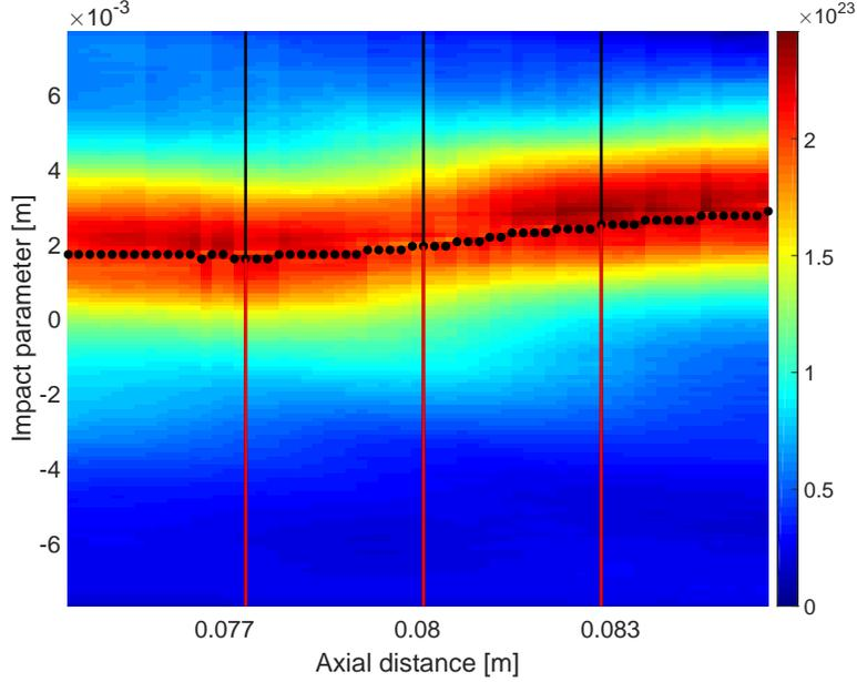
Figure 3.10: The  $n_e$  from Abel inversion of the  $N_e$  in Fig. 3.9(a) using the centroids plotted as black dots. The vertical lines correspond to the profiles plotted in Fig. 3.11.
