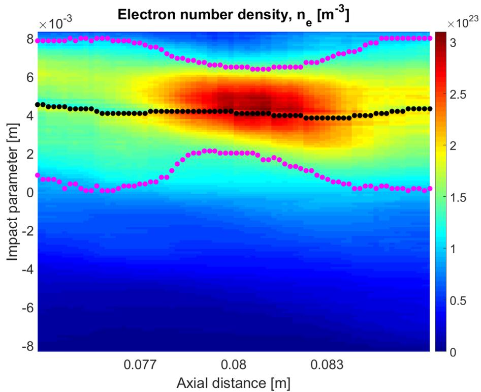
Figure 5.15: Electron number density contour plot showing a sausage mode instability. The DHI image was taken on pulse 160524034 at  $50 \mu\text{s}$ . It shows a  $\lambda \approx 1$  cm sausage mode instability where the plasma size constricts and density increases near  $z = 8$  cm.
