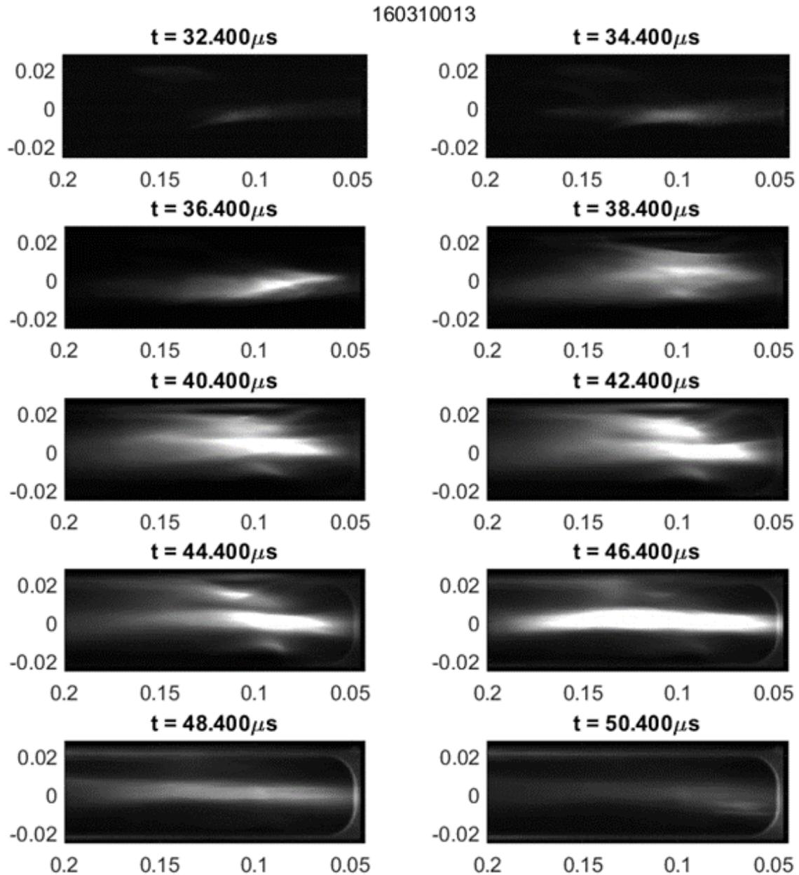
Figure 2.5: Images taken  $2 \mu\text{s}$  apart with the bremsstrahlung bandpass filter installed on the camera lens show a shear flow stabilized Z-pinch between 5 and 20 cm throughout this pulse's quiescent period from 36  $\mu\text{s}$  to 48  $\mu\text{s}$ . The axes are labeled in units of meters relative to the coordinate system of Fig. 2.1.
