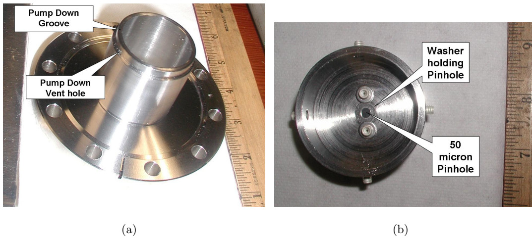
Figure 4.3: Photographs of the EUV plasma shield. (a) The EUV diagnostic shield with a groove cut in the end for a pump down path through the holes drilled in the groove and in the aperture cap. (b) The aperture holds a 50 micron pinhole, which can be replaced by removing the 2 3/4" conflat while leaving the 4 5/8" conflat in place.
