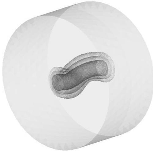
**Figure 16: MH4D screw pinch simulation snapshot showing pressure contours.  $t=0.9 \mu\text{s}$  ( $dx=5 \text{ mm}$ ). For reference,  $\tau_A \approx 0.5 \mu\text{s}$ .**
