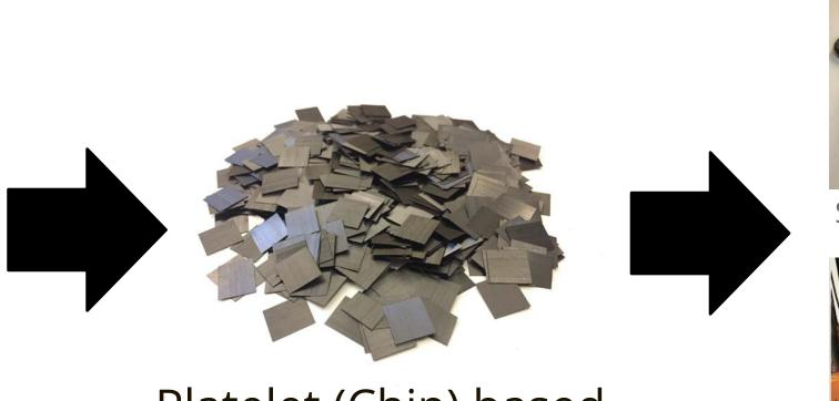
Platelet (Chip) based, discontinuous fiber form
