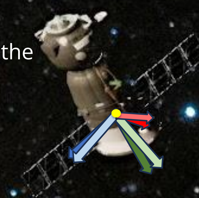
Orientation estimation by neural network on test case of target satellite
