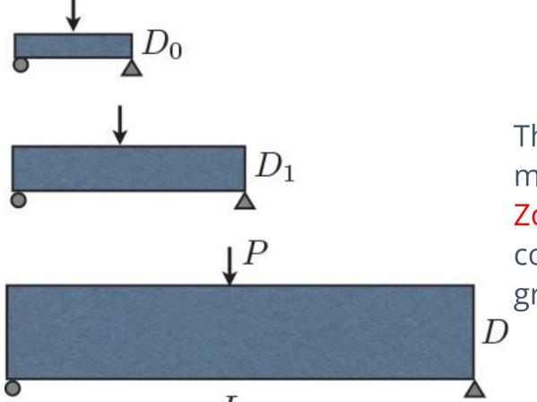
The zone containing strain softening microstructures is called Fracture Process Zone (PFZ). When the size of the structure is comparable to FPZ, the fracture behavior can greatly change.
