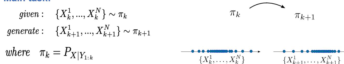
> OTPF approach: update particle with the optimal transport map form  $\pi_k$  to  $\pi_{k+1}$  to  $X_{k+1}^i = T_k(X_k^i)$
