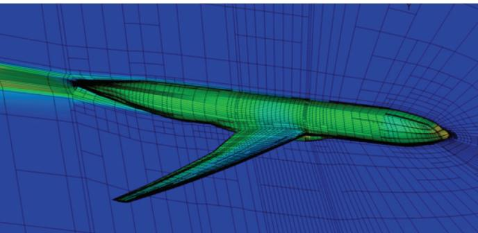
Quantitatively accurate results from realistic Computational Fluid Dynamics (CFD) simulations are often accompanied by high computational expense. Higher-order methods are good candidates for providing accurate solutions at reduced cost. However, these methods are still not robust for industrial applications. In this talk, I will present some of my research work to address this problem.
