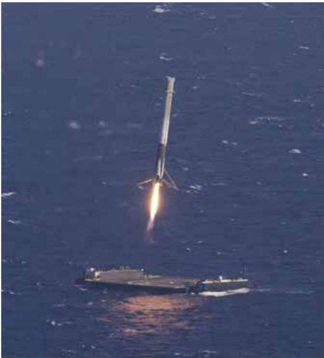
SpaceX's reusable rocket program aims to reduce the cost of space travel by making rockets that can land, refuel and reflly, instead of being thrown away after every flight. Precise landing of a rocket is a unique problem, which has been likened to balancing a rubber broomstick on your hand in a windstorm. Rockets do not have wings (unlike airplanes) and they cannot rely on a high ballistic coefficient to fly in a straight line (unlike missiles).
