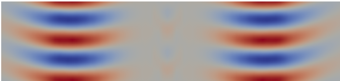
Figure 7.8: Typical WARPM Vlasov-Maxwell simulation result with initialized with equilibrium perturbation adhering to the solution for even mode ‘A’. The image shows the E_y electric field component amplitude.
