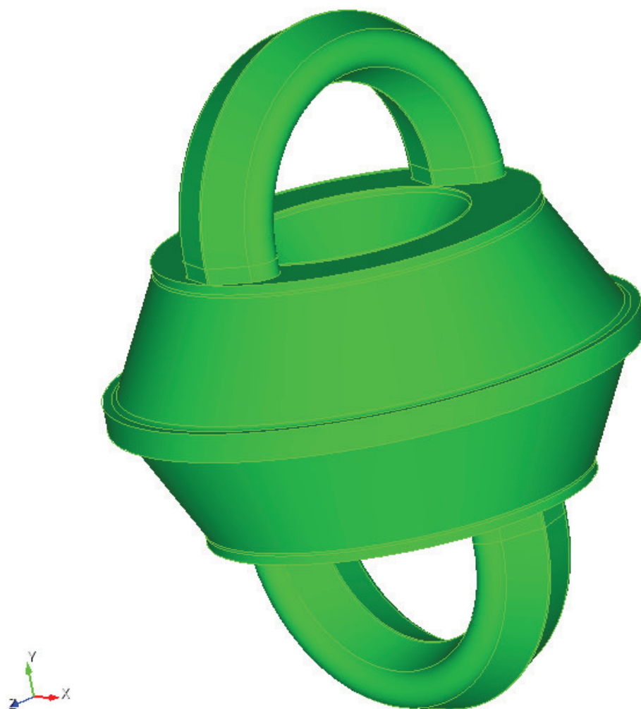
Figure 10.1: Sample CAD file of HIT-SI geometry imported into CUBIT using an ACIS file.
