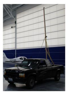
Fig. 29: Stability ground test model mounting system in place in the back of a pickup truck.
