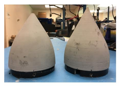
Fig. 19: The nose cone (left) and tail cones (right) which make up the outer shell of the drogue.
