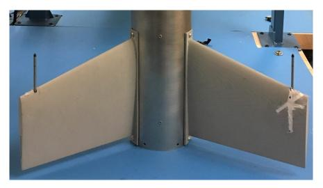
Fig. 20: Two fins with attached pitot static tubes mounted to the fuselage.
