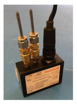
Fig. 14: Honeywell Precision Pressure Transducer.
