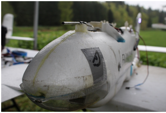
(a) The aircraft with the camera mounted in the nose behind a clear nose cone.
