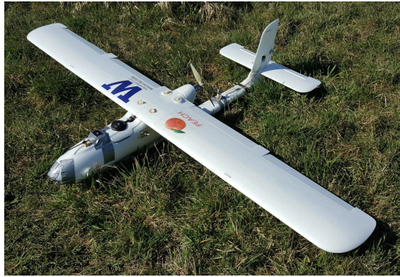
(a) TRAPIS payload integrated onto the Finwing Sabre UAS, showing secondary GPS unit, and transponder antenna mounted to the empennage.
