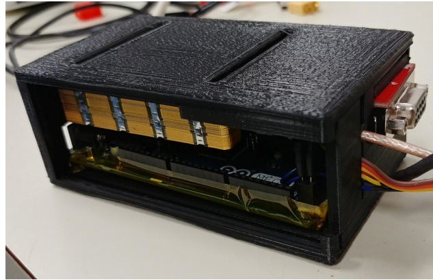
(b) Interior of the payload showing the Arduino and transponder inside the box. Note that this configuration proved unfeasible and was not used in the final flight test.
