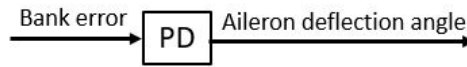
Figure 7. Block diagram showing the flow of signals through the wing leveler component of the WSTR controller.
