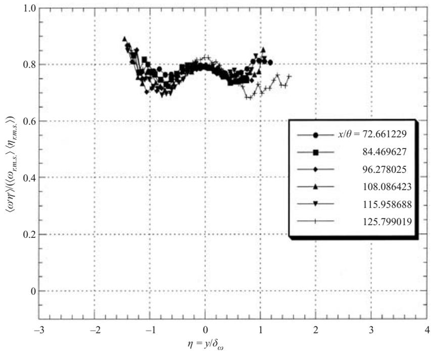
FIGURE 9. Mean vertical conditional vorticity–elevation correlation coefficient profiles at various downstream locations. Only vorticity within the range  $[-15, -1.0]$ , and negative elevation values are correlated.
