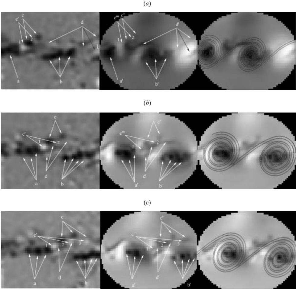
FIGURE 4. Instantaneous vorticity (left) and FSD (centre and right) plot at (a)  $t = 0$ , (b)  $t = 0.267$  s; and (c)  $t = 0.4$  s. The flow is from left to right; the high-speed side is on the top, and low speed side is on the bottom. Each of the images shows an area 22 cm wide by 18 cm high. The velocity ratio,  $U_2/U_1$ , is 0.467, and the vorticity thickness is 4.5 cm. The FSD on the right includes graphically drawn spirals to show the location of the main rollers in relation to the FSD.
