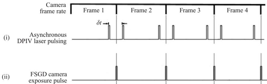
FIGURE 3. FSGD and DPIV timing synchronization diagram.
