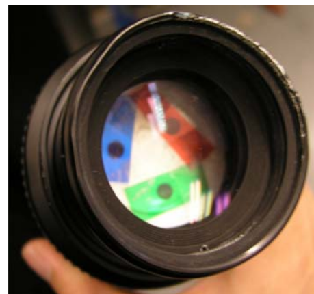
Fig. 2 The three color-filtered pinholes on the aperture mask
