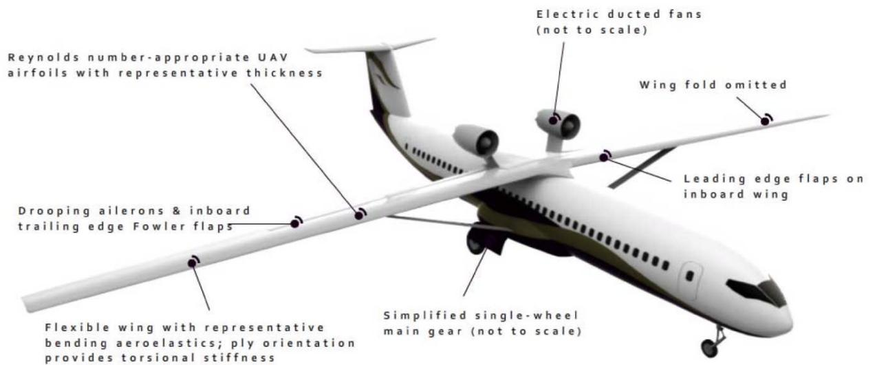
Figure 44: Key elements of the 2011 Strut-Braced-Wing concept UAV.
