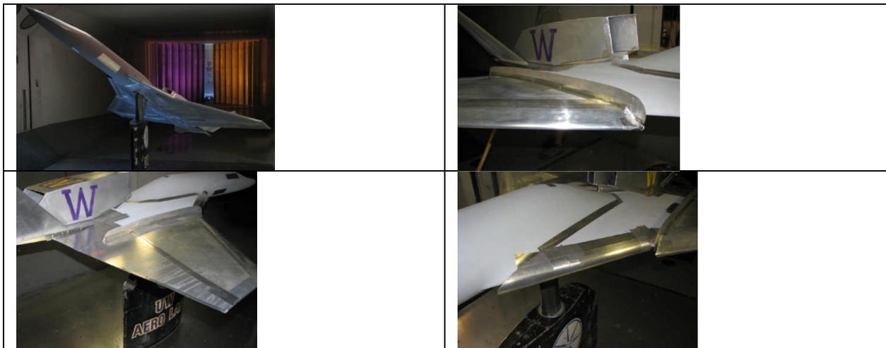
Figure 23: The 2009 wind tunnel model at the Kirsten wind tunnel plus selected applied aerodynamic fixes of the pitch-up problem, including fences, redesigned strake, and rearwards area increase of the inboard wing section.
