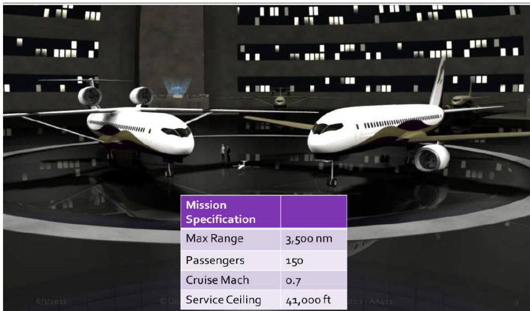
Figure 42: The full size baseline configurations studies in the conceptual design phase of the 2011 project.
