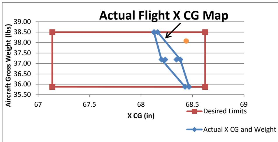
Figure 32: Center of gravity travel for the 2009 UAV.
