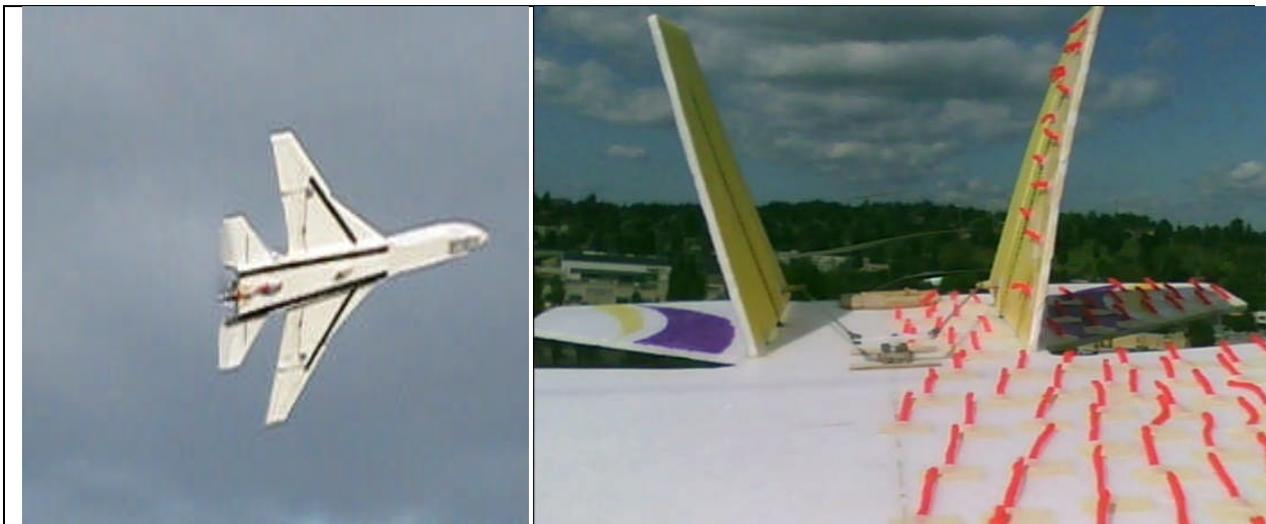
Figure 37: The “2010 “foamie” – a ½ scale avionics systems testbed for the 2010 UAV. On the right – tufts used to study the flow field over the wing during maneuvering flight.
