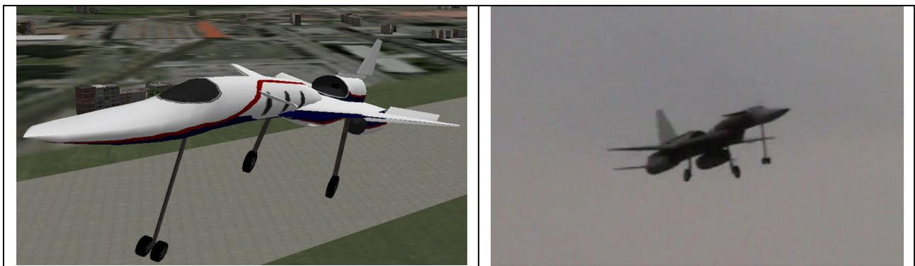
Figure 7: An X-Plane simulation model of the 2006 UAV and the actual UAV in flight.
