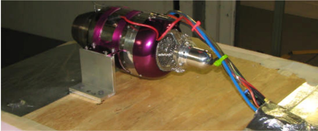
Figure 25: The PST-J800R engine on its test stand.
