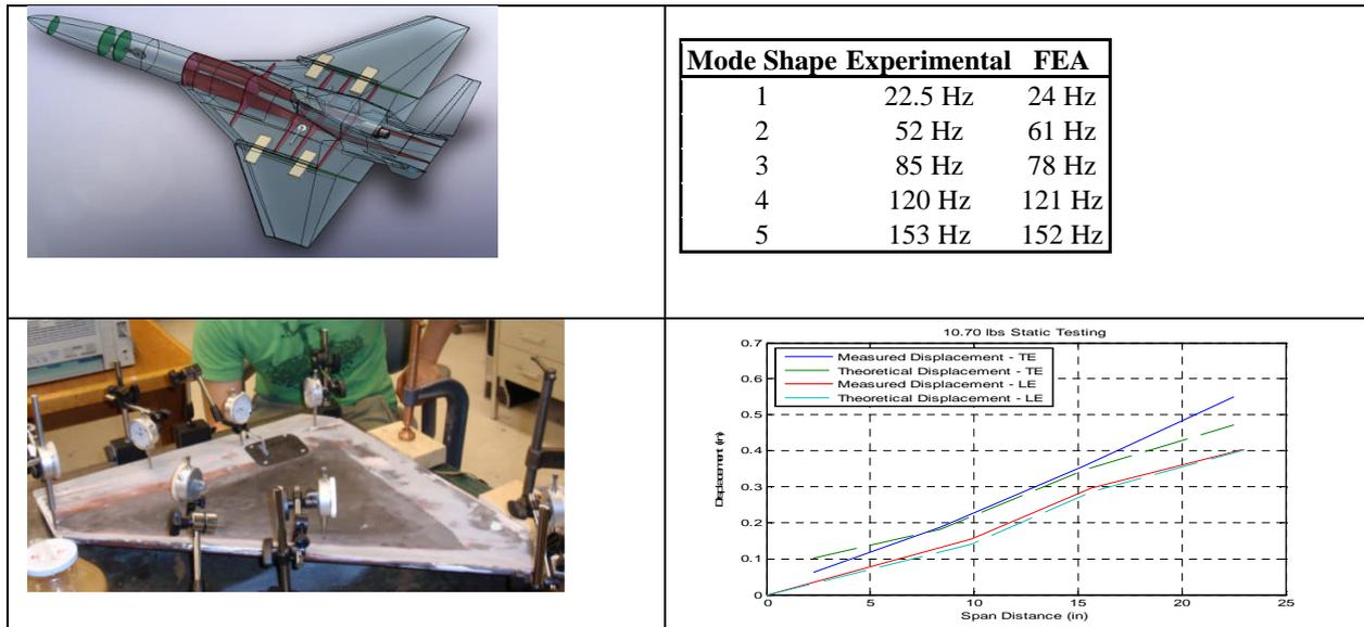
Figure 31: The structural arrangement of the 2009 UAV plus modal and static analysis and test results for the wing's outer panel.
