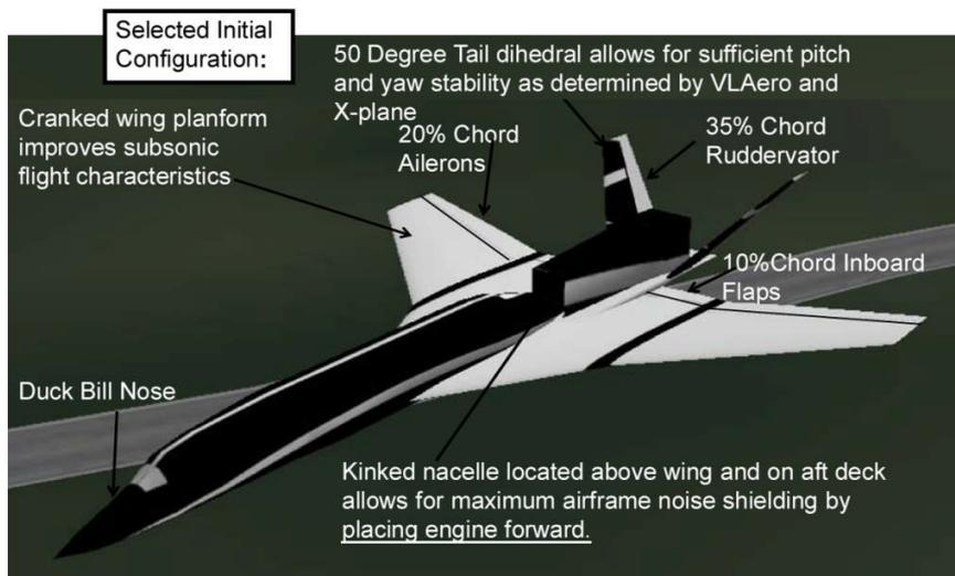
Figure 21: The selected 2009 UAV configuration.
