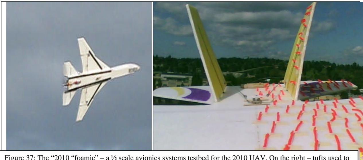
Figure 37: The “2010 “foamie” – a ½ scale avionics systems testbed for the 2010 UAV. On the right – tufts used to study the flow field over the wing during maneuvering flight.
