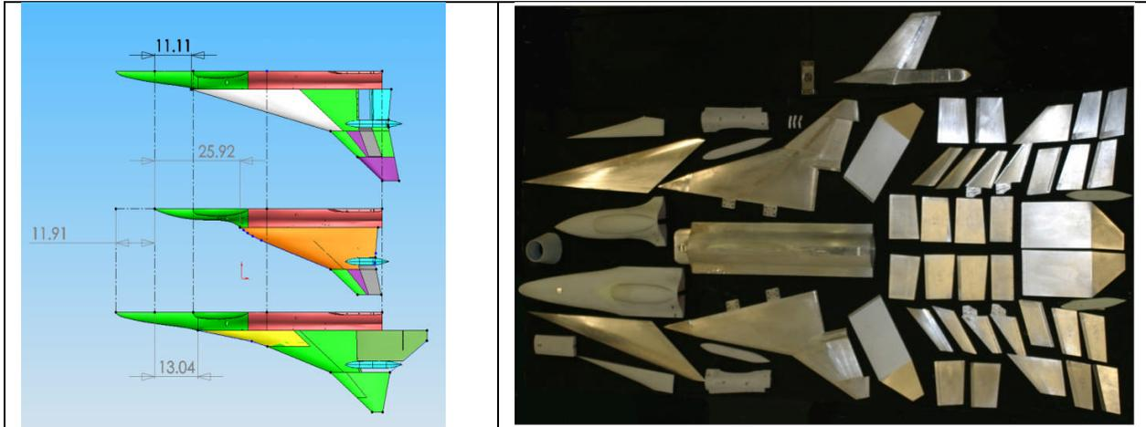
Figure 10: Wind tunnel configurations and models tested at the Kirsten Wind Tunnel for the 2007 capstone airplane design course. Wind tunnel model developed built by Aeronautical Testing Service, Inc., of Arlington, WA.
