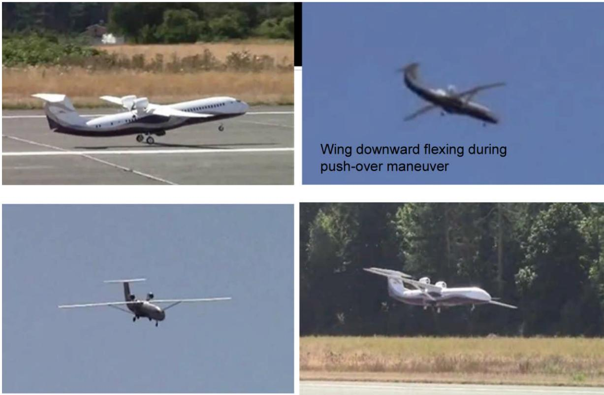
Figure 49: The 2011 University of Washington SBW UAV in flight, Summer 2011.
