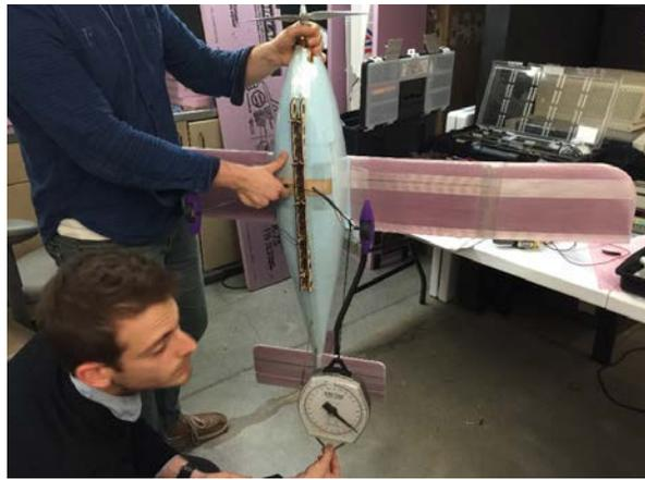
**Figure 7.3:** Landing gear strut testing in the backward direction
