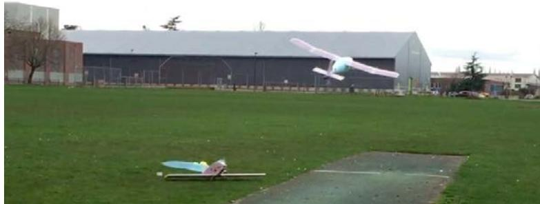
**Figure 8.1:** Prototype 2 climbing on take-off at maximum load
