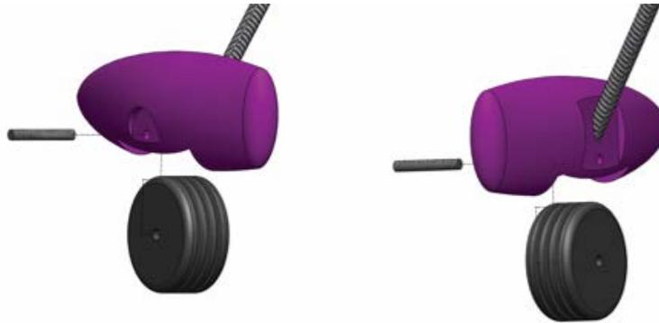
**Figure 5.3:** Landing gear installation
