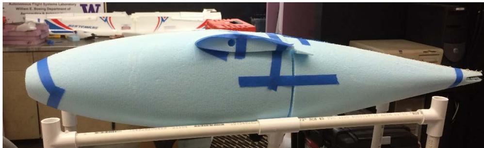
Figure 6.3: CNC-milled fuselage
