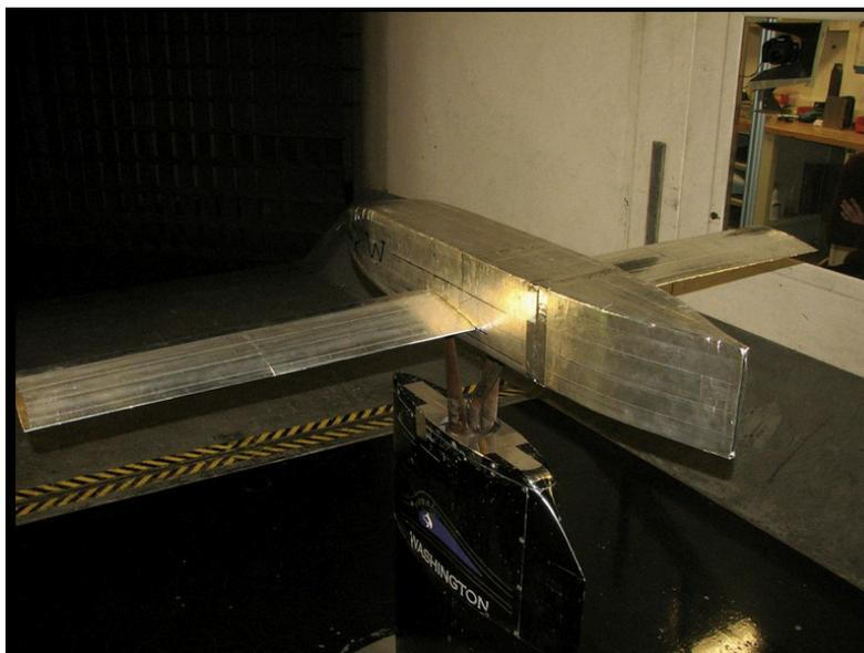
**Fig. 4.5.** A rear view of the model mounted in the Kirsten Wind Tunnel.
