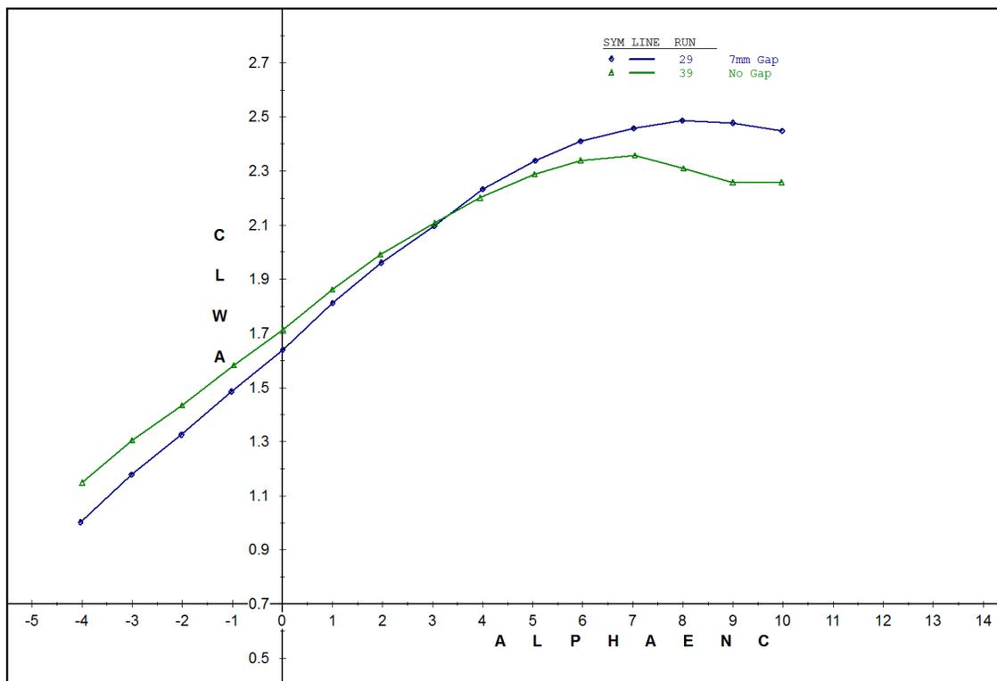
Fig. 4.9. Lift coefficient vs. angle of attack for flap with and without gap.
