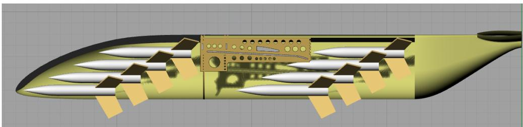
**Fig. 3.2.** Rocket layout within fuselage.
