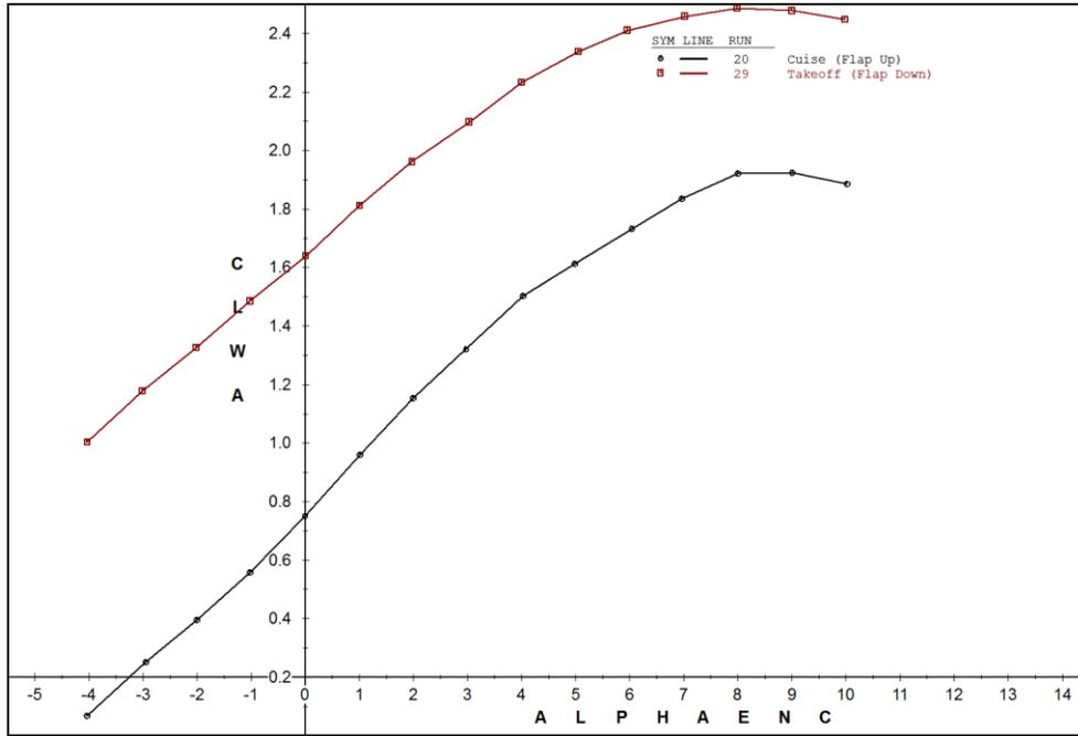
Fig. 4.6. Lift coefficient vs. angle of attack for cruise and takeoff wing configurations.
