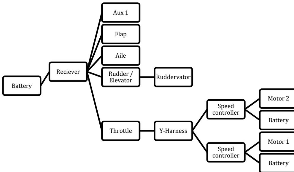
**Fig. 5.1.** Systems Circuit Flow-Chart
