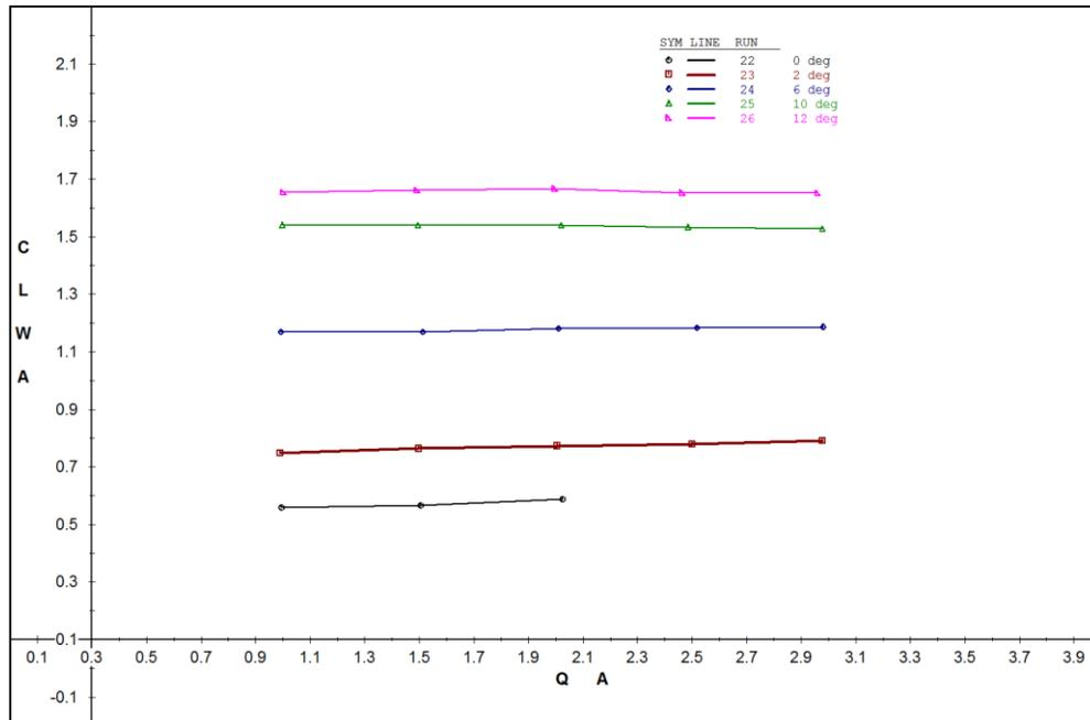
**Fig. 4.5.** Lift coefficient vs. dynamic pressure for varying angles of incidence of the takeoff flap.
