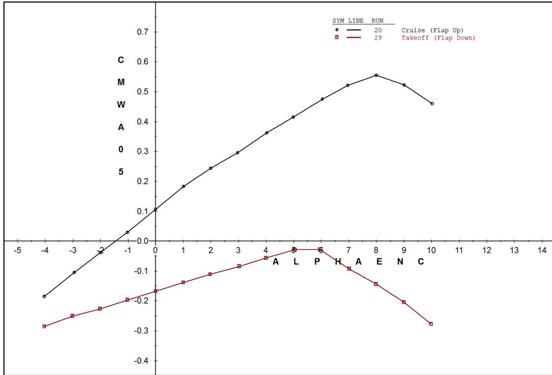
**Fig. 4.8.** Pitching moment vs. angle of attack for cruise and takeoff wing configurations.
