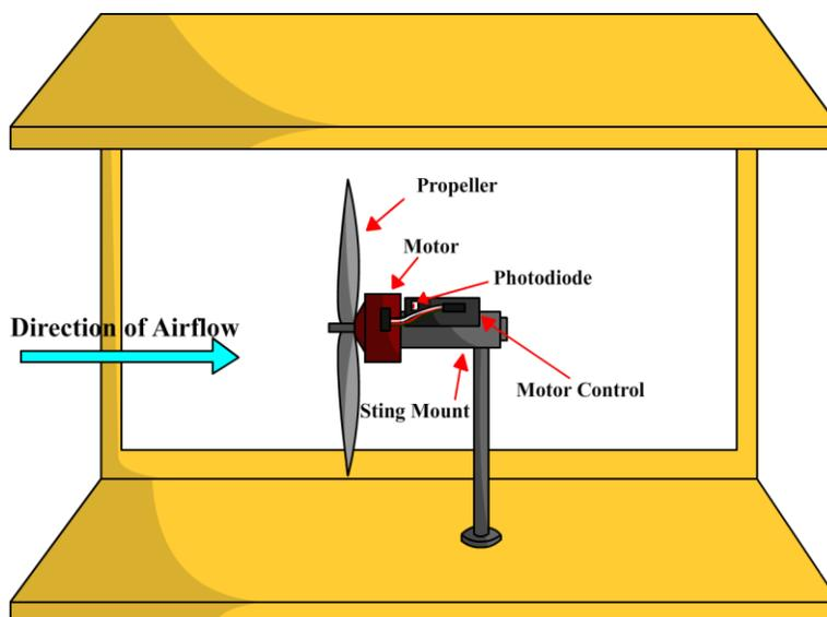
**Fig. 4.1.** Power testing of propeller and motor to determine power available for take-off roll
