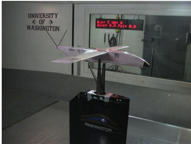
**Fig. 4.2.** Model mounted in the KWT test section.
