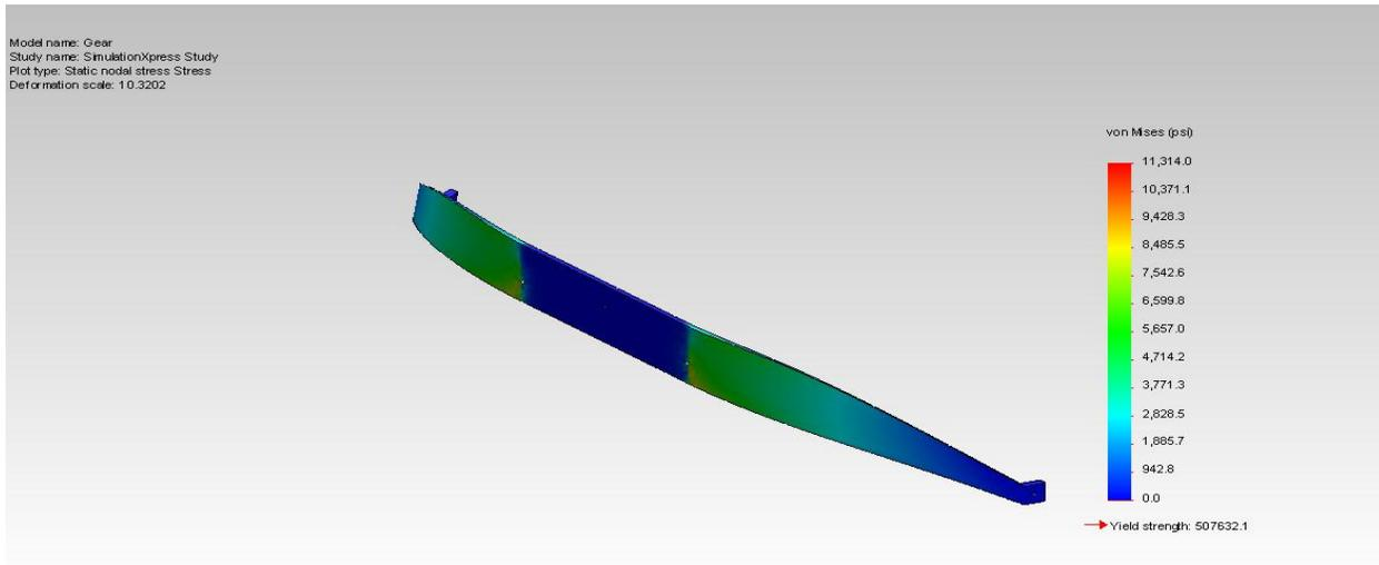
**Fig. 7.1.** Von Mises stress concentrations on landing gear strut.
