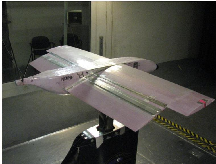
**Fig. 4.3.** Model with flap section deployed.
