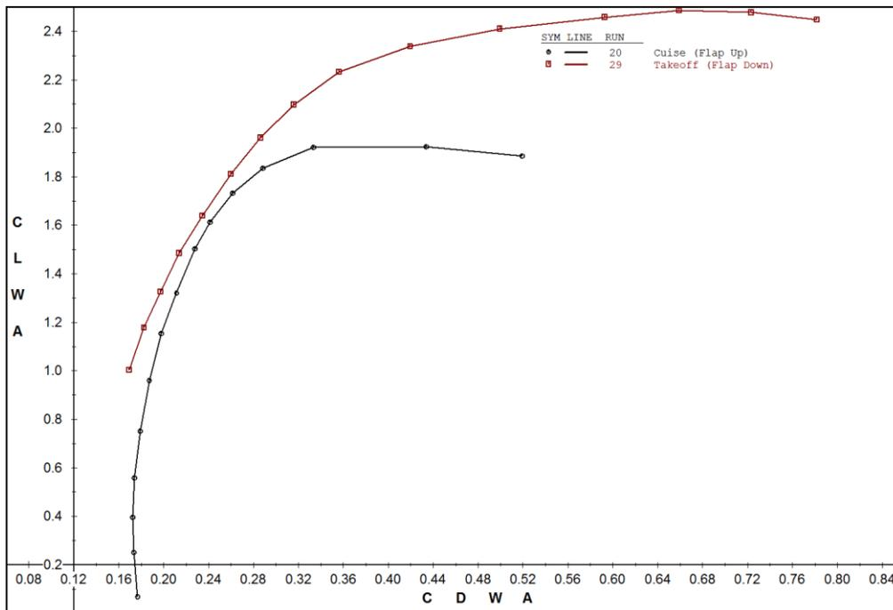
Fig. 4.7. Lift coefficient vs. drag coefficient for cruise and takeoff wing configurations.
