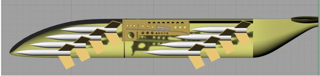
**Fig. 3.2.** Rocket layout within fuselage.
