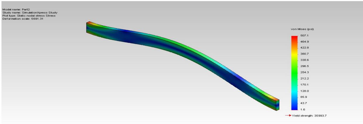
**Fig. 7.2.** Von Mises stress concentration on wing spar.
