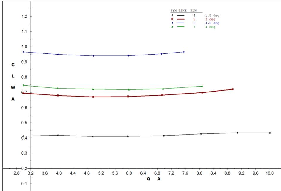
**Fig. 4.4.** Lift coefficient vs. dynamic pressure for varying angles of incidence of the cruise wing.
