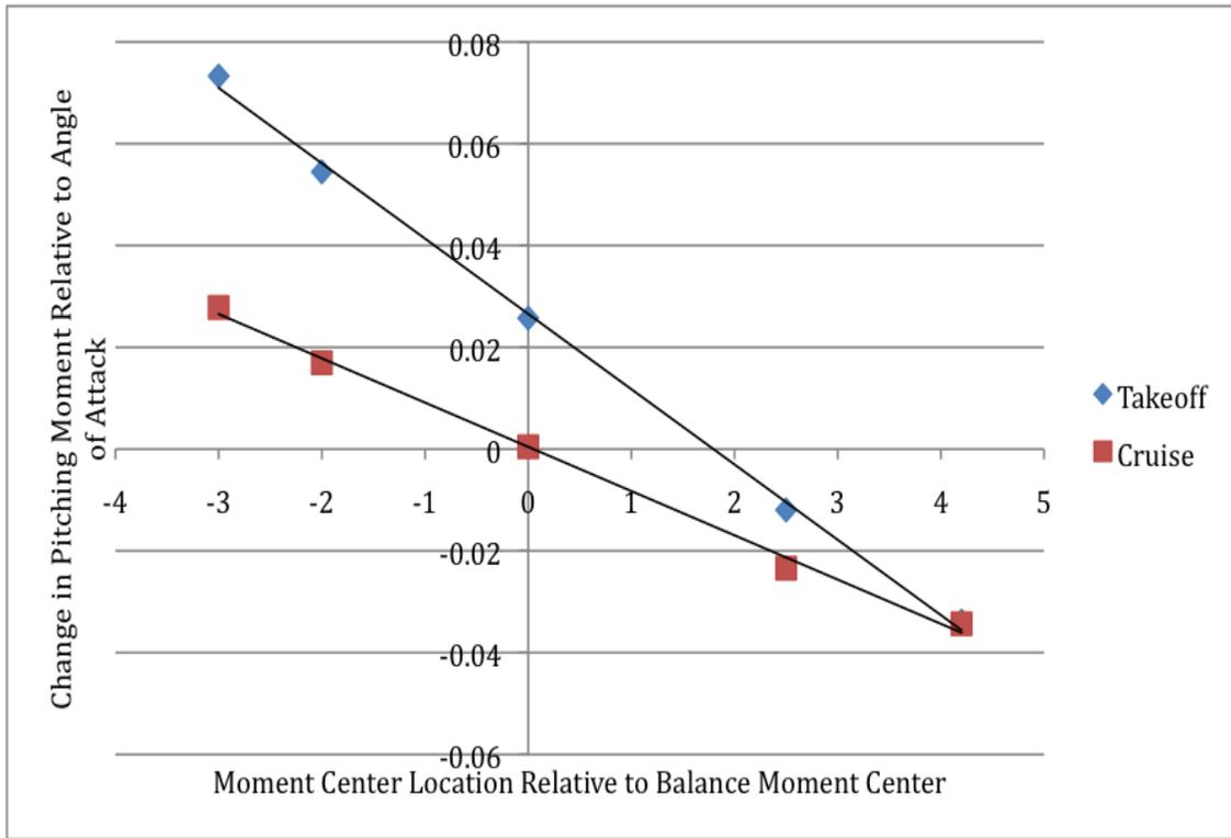
Fig. 4.10.  $\frac{\partial C_m}{\partial \alpha}$  vs. distance from balance moment center.
