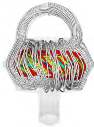
The spheromak concept: the magnetic bottle is the colored region, and the gray edge is the field line.
