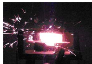
Long-exposure picture of 30,000 Amp strike with incandescent CFRP debris
