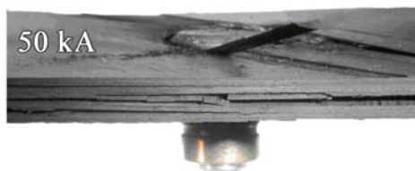
Damaged CFRP specimen with fastener following a 50,000 Amp strike
