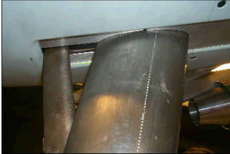
Looking Up at the Underbody Panel and Strut Seal. Model is at the maximum angle of attack.
