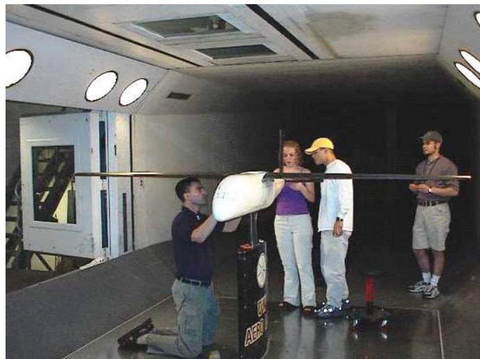
Fig. C.2 Kirsten Wind Tunnel test section with AA 410/411 model and students.
